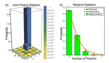
FIG. 3: (a) Joint photon statistics  $p_{n,m}$  measured with two TMDs and pump power of 220nW. (b) Marginal statistics of idler with pump power of 375nW. The measurement is fitted against thermal and Poissonian distributions.
