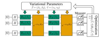
Fig. 1: Sketch of the QAOA-circuit for p = 2.
