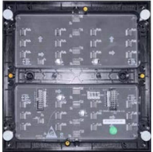
(b) Backside of the LED-matrix with its power supply and pin-layout.
