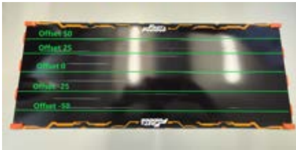
(a) Distinction of the track in Anki Overdrive with discrete offset positions from -50 to +50 with \pm 25 steps.
