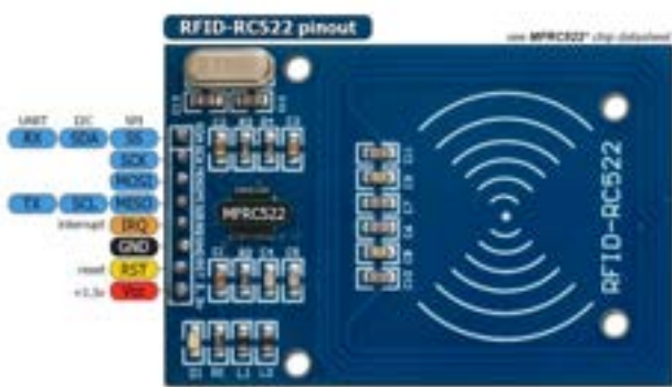
(a) MFRC522 RFID-module pin-layout [50].
